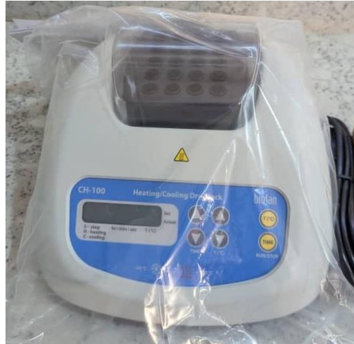
Heating/Cooling Dry Block
